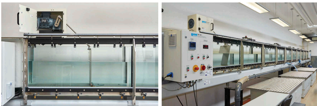
Figure 2. Flap-type wavemaker and the experimental flume in the Hydraulic Laboratory of the Faculty of Civil Engineering at the University of Rijeka.
